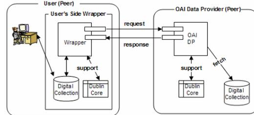
Fig. 5 P2P-based Harvesting with user's side wrapper
