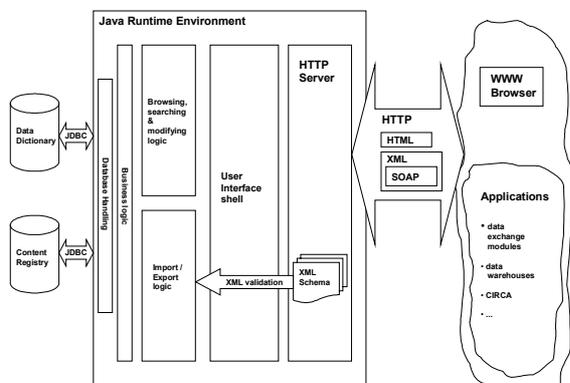
Figure 6: System Architecture
