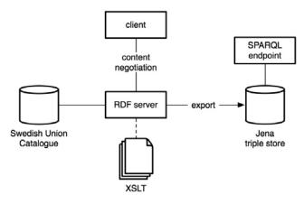
FIG. 1. Implementation schematic
