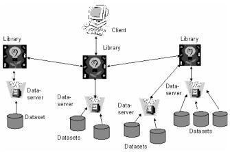
Figure 1. Deployment of the MISSION system
