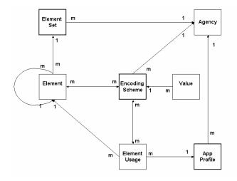
**Figure 1:** The base registry data model
