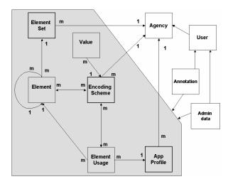
**Figure 3:** The extended registry data model
